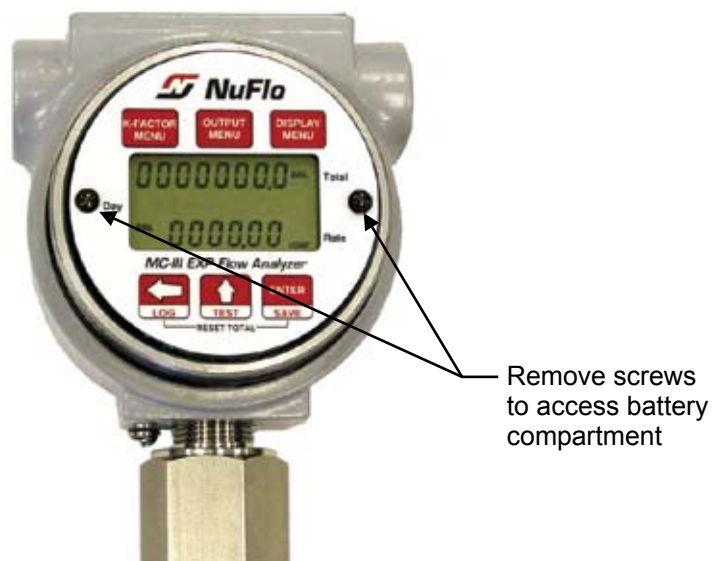
Figure 6.1— Removal of faceplate/keypad assembly
