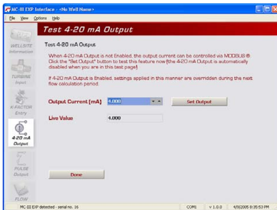
Figure 4.30—4-20 mA output test screen
